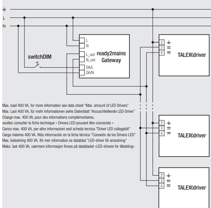
**UK** ready2mains enables digital information to be transmitted via the mains cable with the aid of phase control. The procedure used ensures robust interference-free communication.
