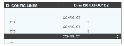
When you have finished configuring the entire load (L1) (type of load, name, rated current, all configured transducers), set the following loads (L2, L3) from the "OUTPUT" line:
