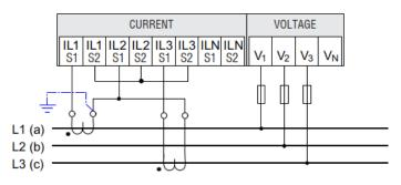
(4) Three-phase measuring, three conductors, balanced load, without voltage transformers, with one current transformer.
