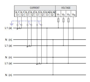
(9) Single-phase measuring, two conductors, with voltage transformers, with three current transformer.
