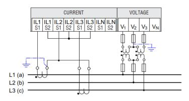
(5) Single-phase measuring, two conductors, without voltage transformers, with one current transformer.
