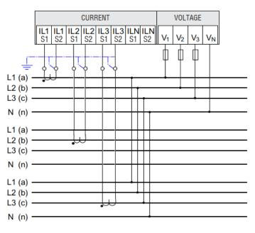
(7) Single-phase measuring, two conductors, without voltage transformers, with one current transformer.
