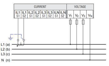
(6) Three-phase measuring, four conductors, balanced multiple loads, with three current transformers.
