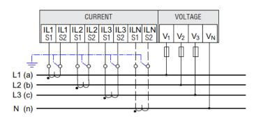
(3) Three-phase measuring, three conductors, unbalanced load, with voltage transformers, with two current transformers. (ARON)
