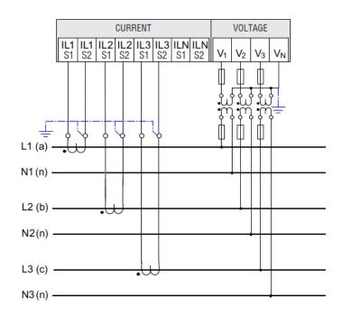
(8) Two-phase measuring, three conductors, unbalanced loads, without voltage transformers with two current transformers.
