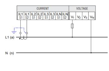
(2) Three-phase measuring, three conductors, unbalanced load, without voltage transformers, with two current transformers. (ARON)
